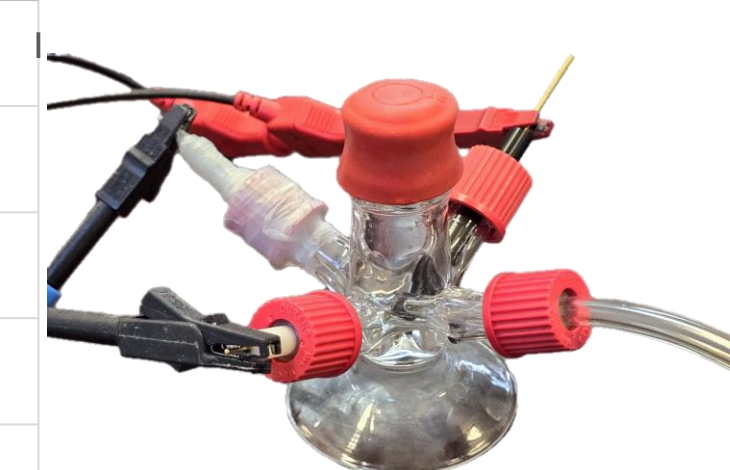
Fig 5. a) Cyclic voltammogram of [Hdema][TfO], b) Photo of 3-electrode set-up (Pt WE, Pt CE, Ag wire RE)
