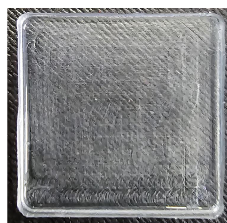
Fig 3. Casted composite membrane with 55 wt% PIL
